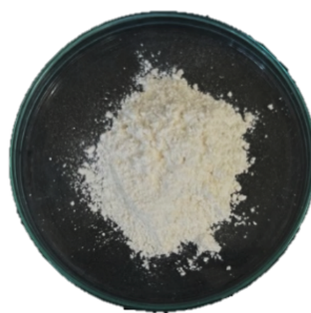
Figure 1. Characteristic of powder of B. amyloliquefaciens strain C2-1 after spray drying at constant 90 °C inlet temperature.
