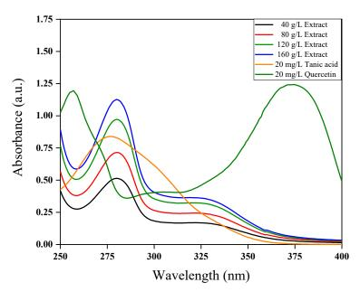
Figure 2. UV-Vis spectra of extract dyes from mangosteen leaves at different concentrations.
